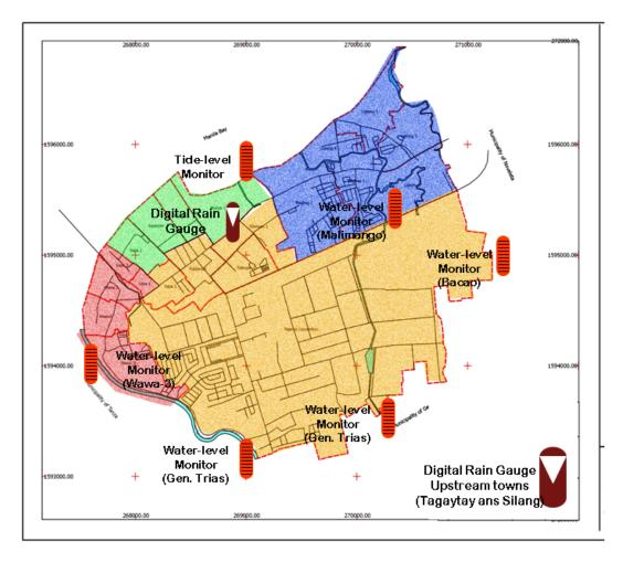
The digitial rain gauge will monitor the amount of rainfall that Rosario receives in any given time. Alarm will be raised whenever the rainfall reaches 40 millimeters within 4 hours as this is categorized by PAGASA as an abnormal heavy rainfall already. The tide monitor installed along the coastline of Muzon
