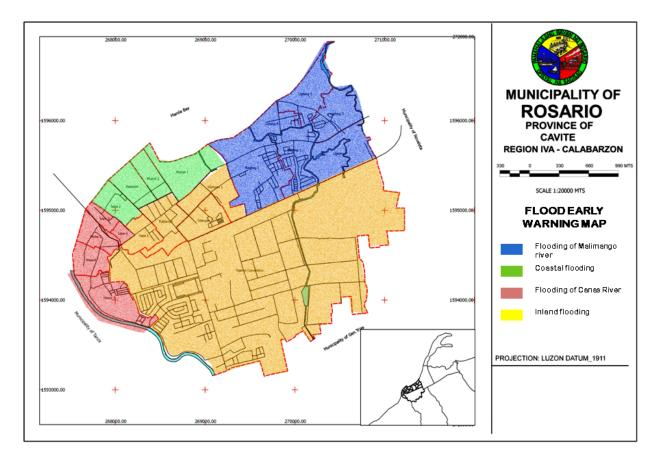
Cluster 1: Areas located along the Canas River. These barangays are flooded whenever the Canas River overflows and caused by heavy rainfall upstream and downstream and complicated by high tide which reduced drainage rate.
